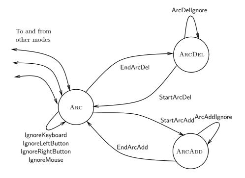
Figure 5.5: X-machine-let showing the replacements for ARC
