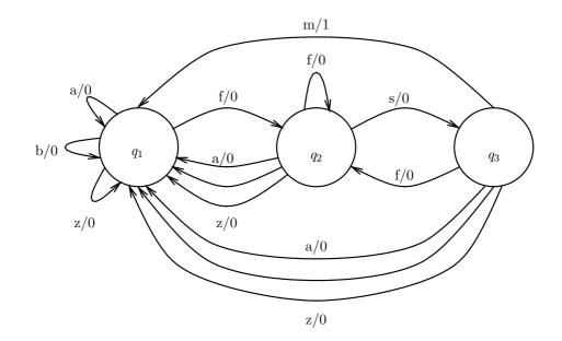
Figure 3.1: State transition diagram of a finite-state-machine to recognise the sequence "fsm".
