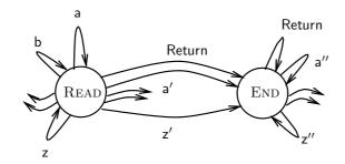
Figure 4.1: A simple X-machine, for entering a text string
