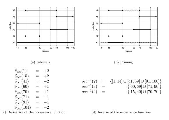
Figure 3: Execution of Algorithm 1: A set of intervals (a). The same set of intervals where inconsistent sub-intervals for a lower bound on the number of equalities of 4 (N'  $\geq$  4) are represented as dashed lines (b). (c) and (d) represent the derivative, and the inverse of the occurrence function for the initial set of intervals, respectively.
