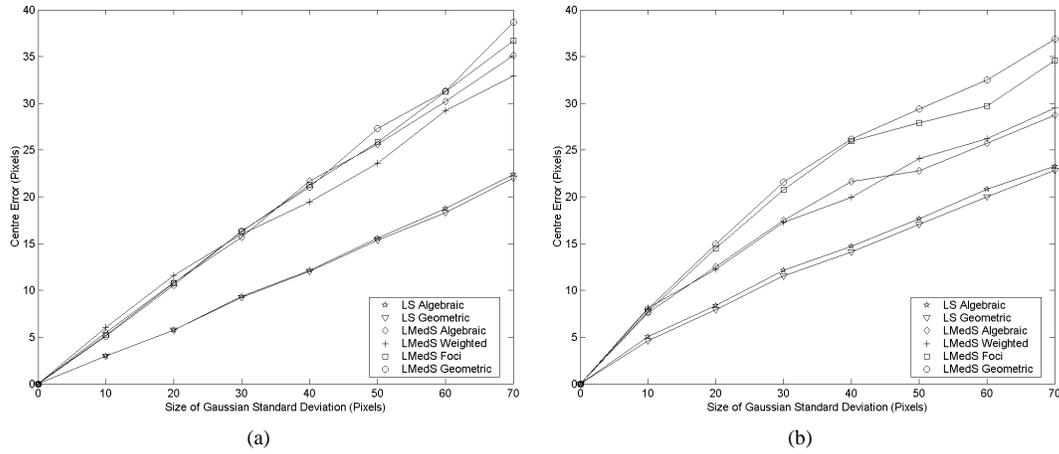
**Figure 4.** Alpha trimmed mean ( $\alpha = 0.1$ ) (a) centre error of less eccentric ellipse synthetic data (b) centre error of more eccentric ellipse synthetic data when Gaussian noise is applied with varying  $\sigma$
