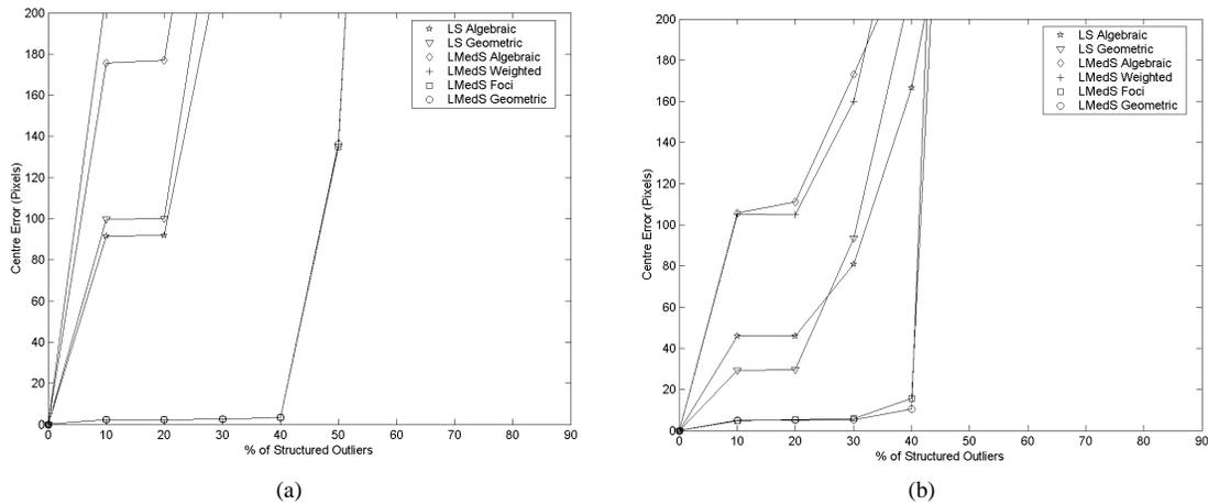
**Figure 6.** Alpha trimmed mean ( $\alpha = 0.1$ ) (a) centre error of less eccentric ellipse synthetic data (b) centre error of more eccentric ellipse synthetic data when structured outlying noise is added
