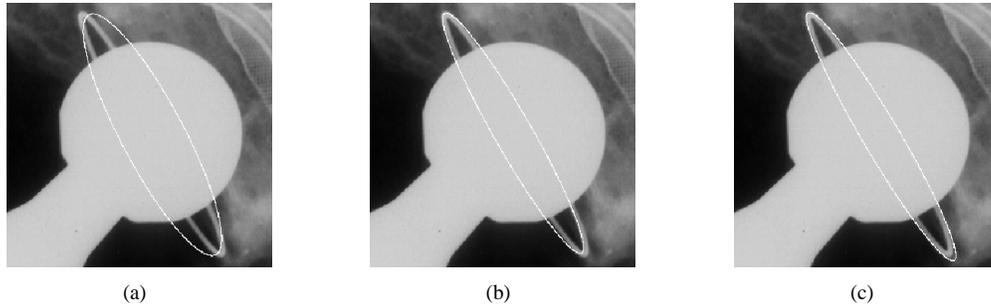
**Figure 7.** Sample eccentric rim with (a) LMedS Algebraic fit (failure) (b) LMedS Foci Fit (success) (c) LMedS Geometric Fit (success)
