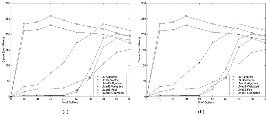
**Figure 5.** Alpha trimmed mean ( $\alpha = 0.1$ ) (a) centre error of less eccentric ellipse synthetic data (b) centre error of more eccentric ellipse synthetic data when mixed Gaussian noise is added
