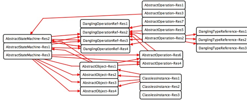
Fig. 11. Conflict graph generated by AGG showing all conflicting resolutions , i.e., mutual exclusions between resolution rules for distinct design defects. In order not to clutter the figure, mutual exclusions between different resolution rules of the same defect have been omitted.
