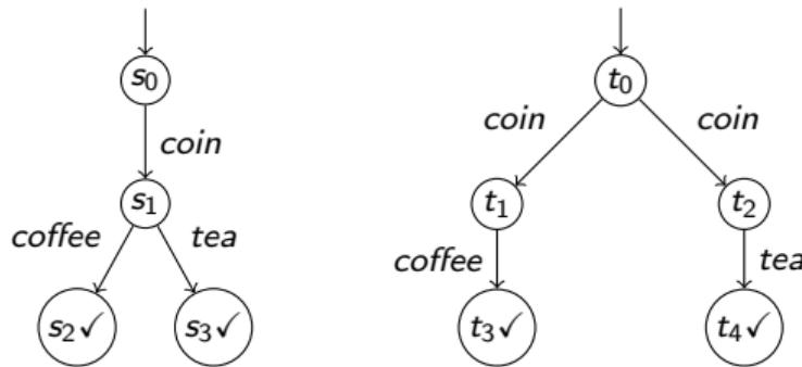
$$Traces(s_0) = Traces(t_0) = \{\epsilon, \text{coin}, \text{coin coffee}, \text{coin tea}, \text{coin coffee}\checkmark, \text{coin tea}\checkmark\}$$
