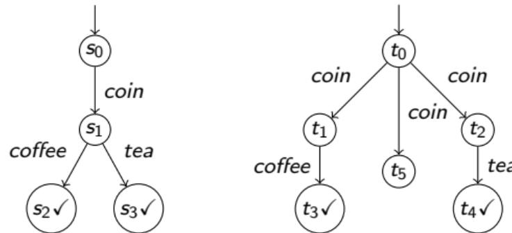
$$\text{Traces}(s_0) = \text{Traces}(t_0) = \{\epsilon, \text{coin}, \text{coin coffee}, \text{coin tea}, \text{coin coffee} \checkmark, \text{coin tea} \checkmark\}$$
