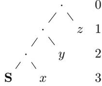
The distance  $d(M, N)$  between two terms is defined as  $2^{-n}$  where  $n$  is the length of the shortest common position  $p$  of  $M$  and  $N$  such that  $M$  and  $N$  differ at  $p$ . With this notion of distance the set  $\mathcal{CL}$  of finite terms becomes a metric space and  $\mathcal{CL}^\infty$  its metric completion.
