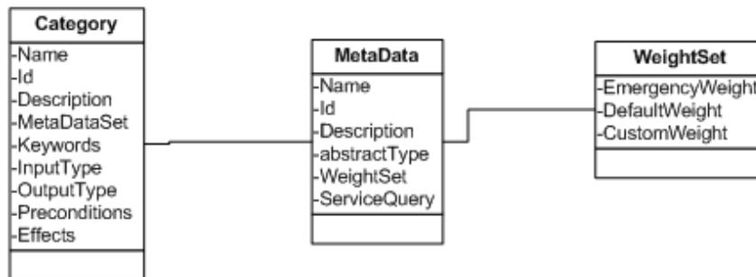
Figure 3.8: The conceptual model of MetaData
