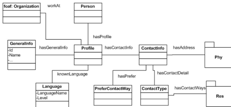
Figure 3.2: User profile package UML diagram
