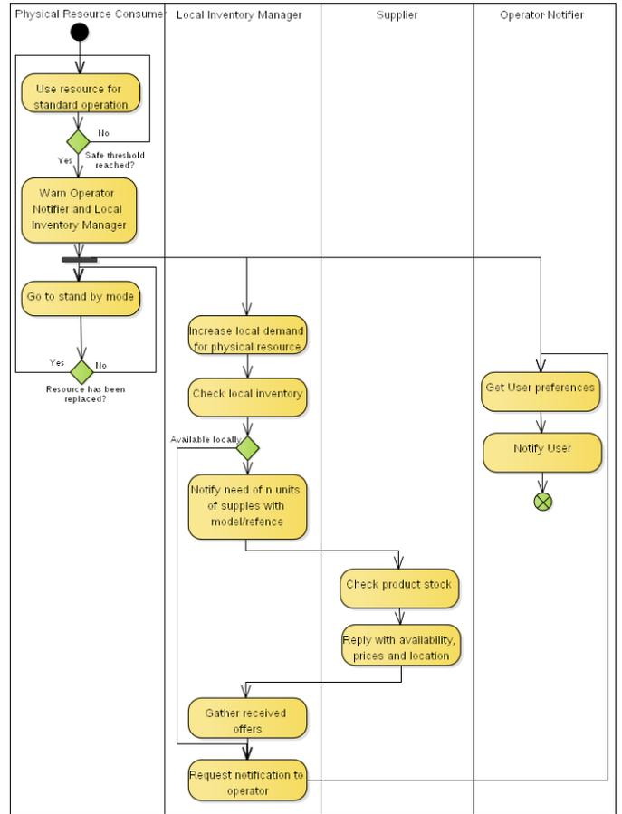
Fig. 3. Scenario for Physical Resource Provisioning
